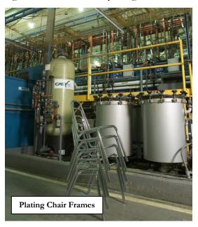
is added to the system only to make up for evaporation from the tanks. Columbia is now exempt from air and water discharge permits and from hazardous waste treatment permits (RCRA-TSD) because of the integral zero-discharge system.
